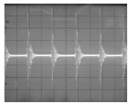
**Image 2:** Amplifier A, Common Mode. 500ns/div, 1V/div.
