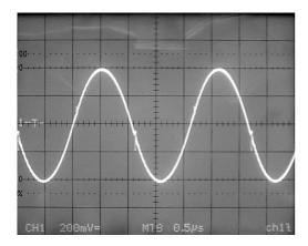
Image 3: Amplifier B, Differential Mode. 500ns/div, 200mV/div.
