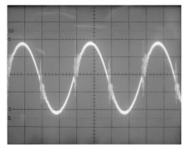
**Image 1:** Amplifier A, Differential Mode. 500ns/div, 200mV/div.
