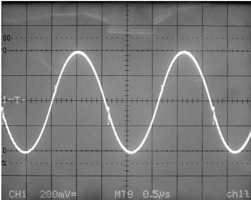
**Image 3:** Amplifier B, Differential Mode. 500ns/div, 200mV/div.
